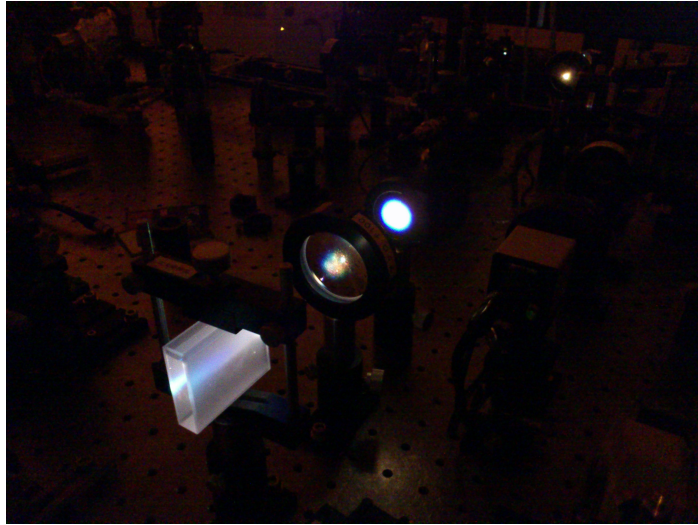
Figure 13. White light is emitted by focusing the creation laser in the quartz cell filled with water.
