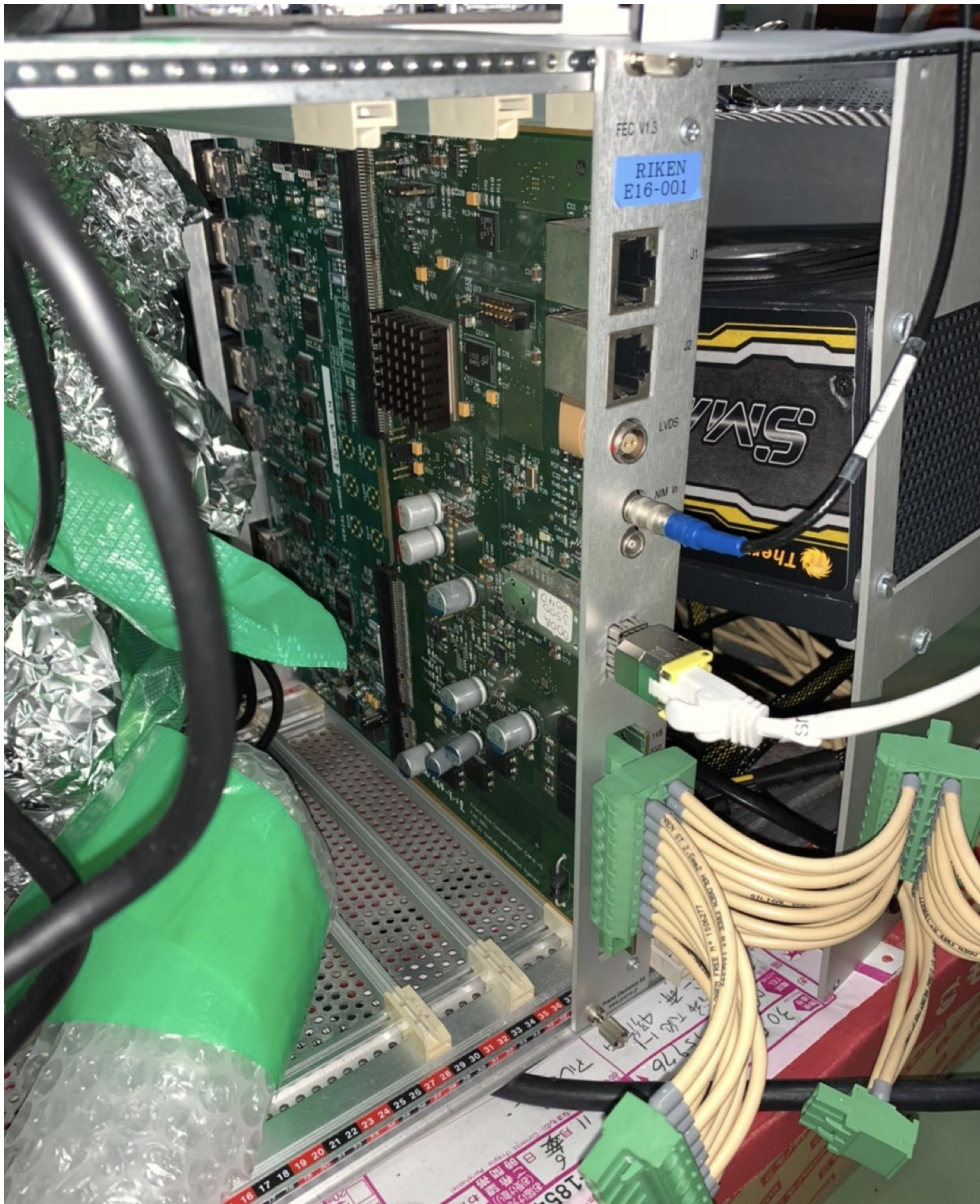
Figure 1.19: Photograph of the SRS. The rear section of the crate contains the ADC card, while the FEC card is visible at the front.
