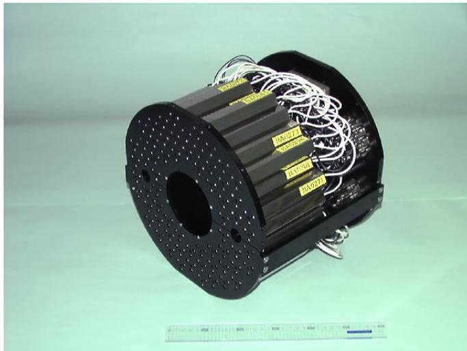
Figure 2.5: A picture of BBC array comprising 64 BBC elements [16].
