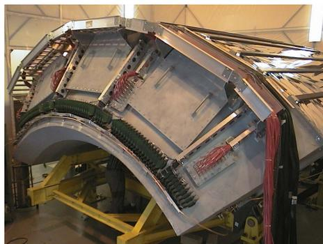
Figure 2.7: The Ring Imaging Cherenkov detector (before an installation)
