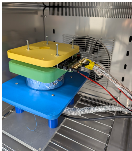
(b) Inside view of the constant-temperature bath showing the AC-LGAD and MCP-PMT mounted on the test bench.
