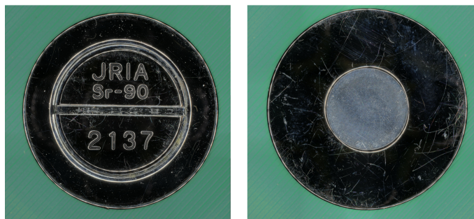
Figure 3.2: Photograph of the ^{90}\text{Sr} beta source used in the experiment. The source emits high-energy electrons that mimic MIP-like events for sensor characterization.
