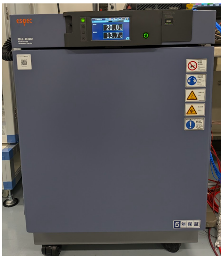
(a) Outside view of the constant-temperature bath housing the AC-LGAD and reference detector.
